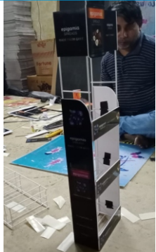
(Sun Board Supporting With Iron Wire)
